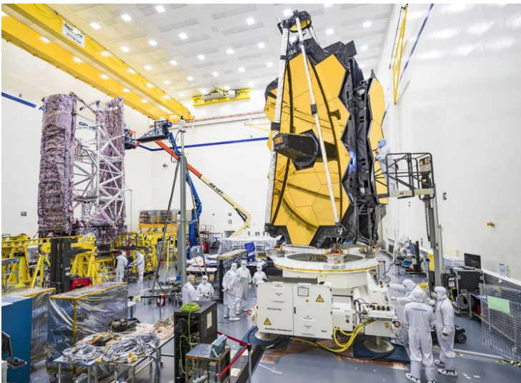
Webb telescope with mirror assembly folded for launch
