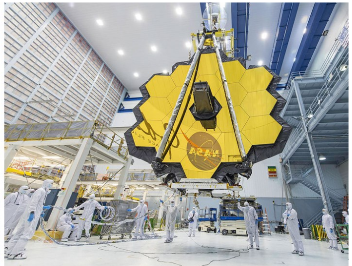
Webb telescope with mirror assembly deployed as in space
